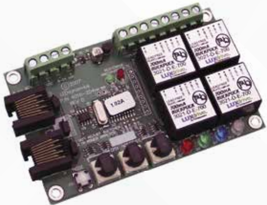
The 4016 QuadPuck LED Driver Interface with (4) 3021-D-E-0700 BuckPuck Drivers (drivers sold separately).
