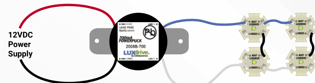
PowerPuck 2008B-700 driving (4) Cree™ or Luxeon™ LEDs from 12VDC.
