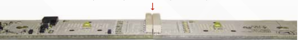
Figure 1 (6) CREE XP-G LEDs in series (V = 24VDC) and end-feeding another strip
