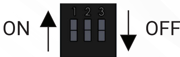
Figure 2. ON/OFF operation of the switch
